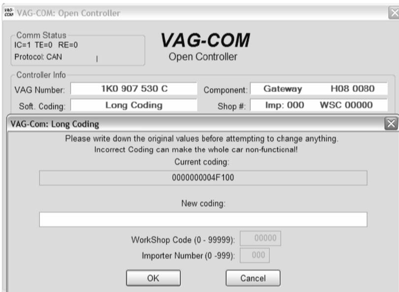
◀ Long Coding. This function is needed to Code some control modules (especially Gateways) in the newest cars. Due to the complexity of Long Coding strings (up to 255 bytes of hexadecimal data) we've accommodated (and urge) the use of Copy & Paste in this function:
