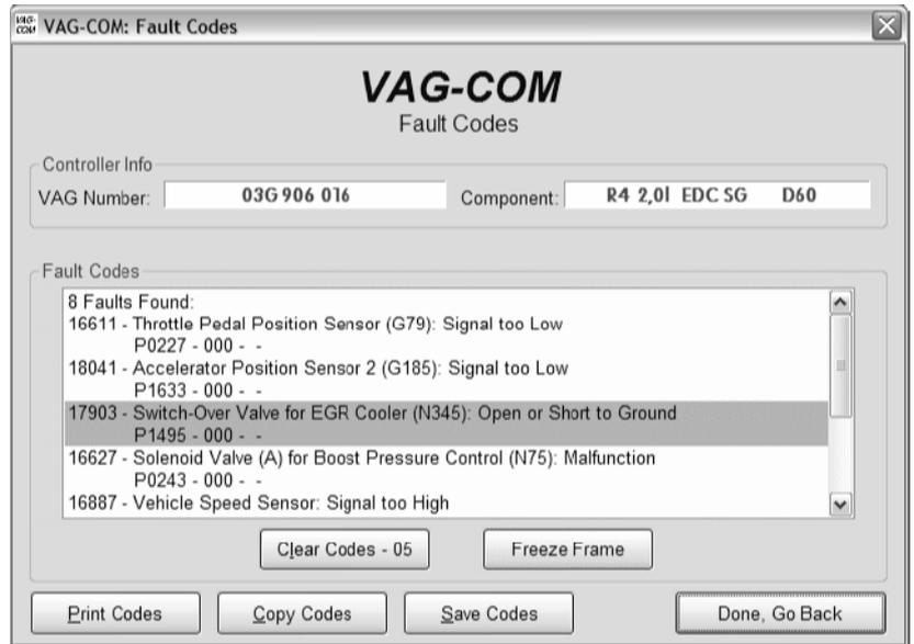
**[Print Codes]** will print a Fault Code Report. If your PC is not connected to a printer when this button is pressed, be sure to use Windows to set the printer to "Work Off-Line" first! Later, when you connect the PC to a printer, un-check "Work Off-Line" to print the report.
