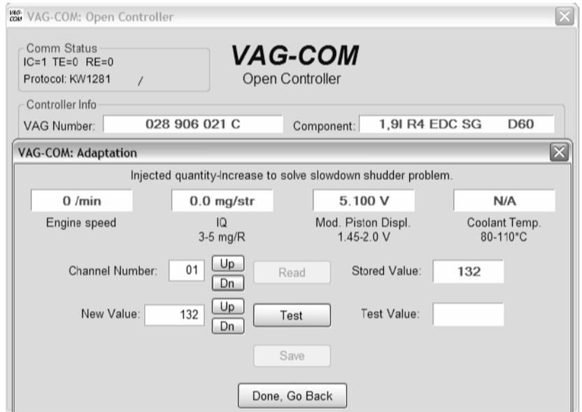
You can use the **[Up]** and **[Dn]** buttons next to *Channel Number* to scroll through all 99 possible channels, or you can manually enter a channel number and click **[Read]**. If a channel exists, VAG-COM will show you the *Stored Value*. If a channel does not exist, the *Stored Value* will show as "N/A". Other data the controller may or may not send will be decoded and shown in the four display fields at the top of the screen.
