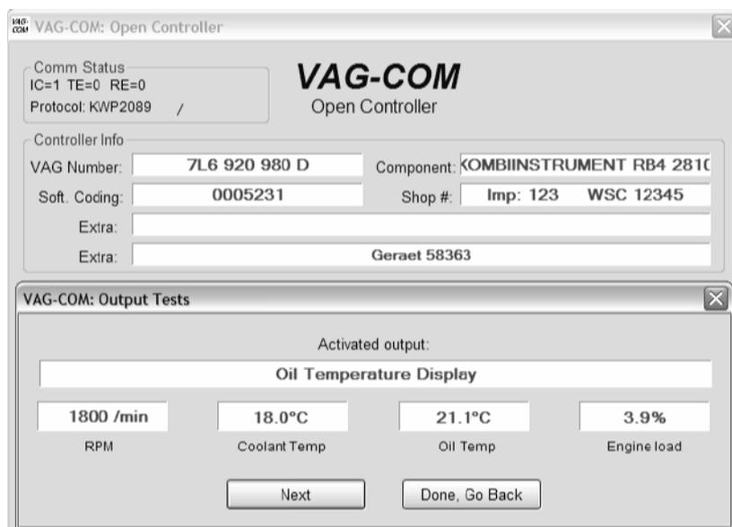
Most Control Modules will permit the Output Test Sequence to be run only one time per session. If you run the Test Sequence to completion, VAG-COM will allow you to return to the previous screen without closing the session, but you may not be able to run the Output Test Sequence again. If you need to run the Sequence again, manually Close the Controller and re-start the session. On some cars, you must cycle the key OFF and ON or even start the engine (to clear the cylinders of fuel).
