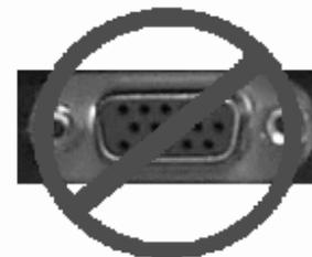
Observe the port we surrounded with the **GREEN** oval. Notice the 9 **MALE** pins? That is a SERIAL port and WILL work! Observe the port circled and crossed in **RED**. Notice the 15 **FEMALE** pins? That is a **MONITOR** port and will NOT work!
