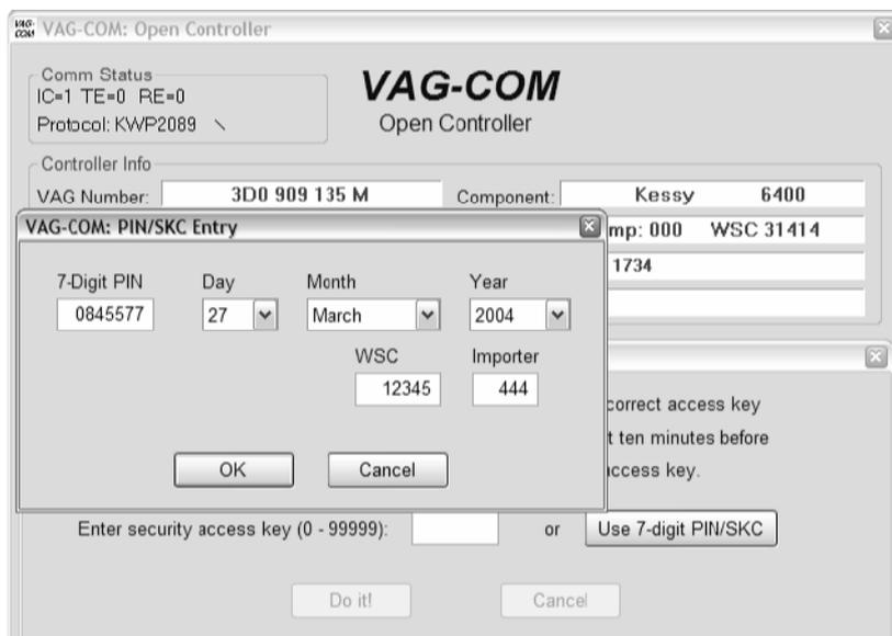
◀The Security Access Function supports 7-Digit SKCs. This is needed for Immobilizer Functions (such as key programming) on the latest vehicles like the Touareg:
