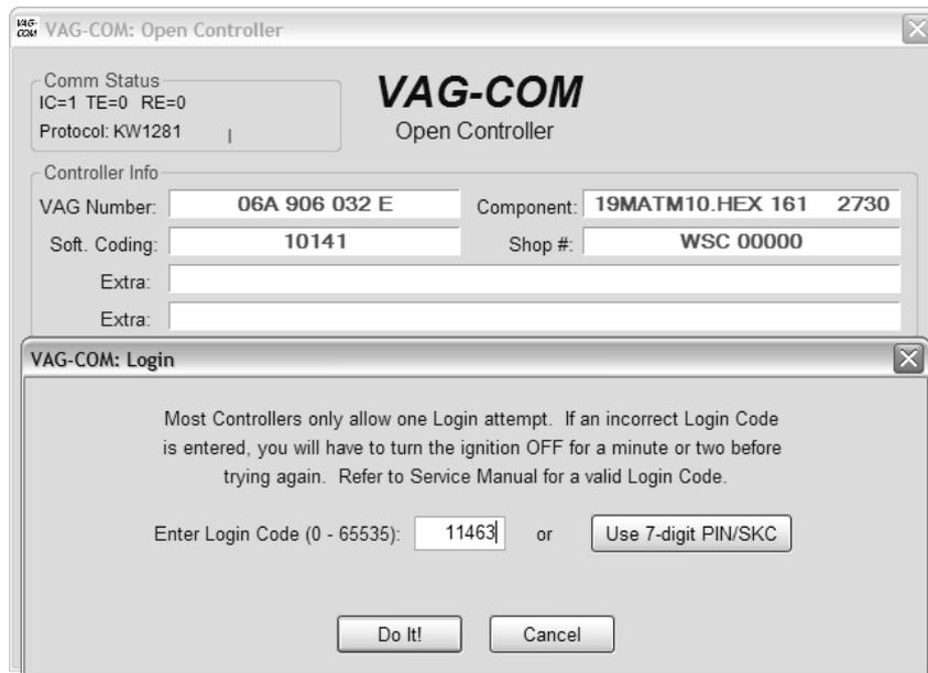
The Login Function must be used on some (but not all) Control Modules before you can Recode or change Adaptation values. On others, it "enables" certain features like cruise control. Valid Login codes can be found in the Factory Repair Manual for your car. If working on an Immobilizer, select **[Use 7-digit PIN/SKC]** to enter a 7-digit Secret Key Code. This function is described in the SKC section of this manual.
