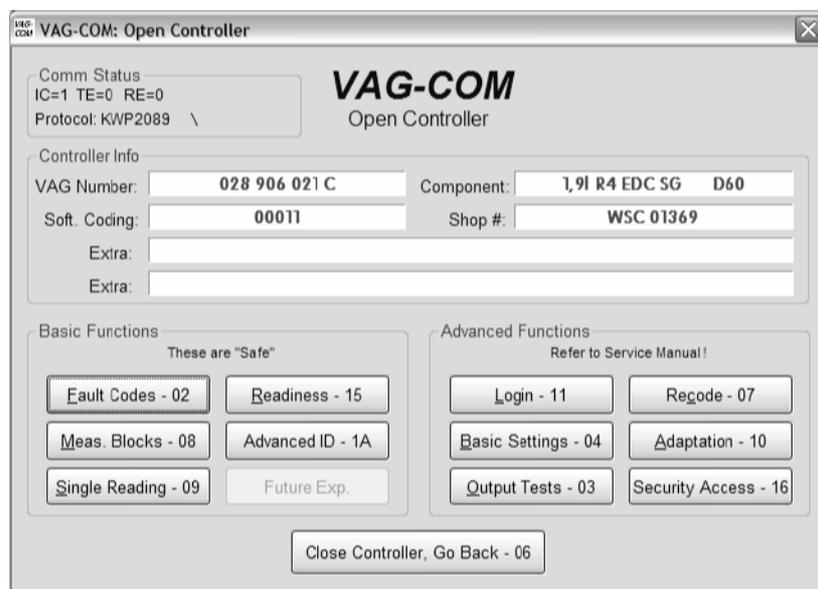
This screen will appear when VAG-COM is attempting to establish communications with any of the Control Modules shown on the Select Control Modules Screen.
