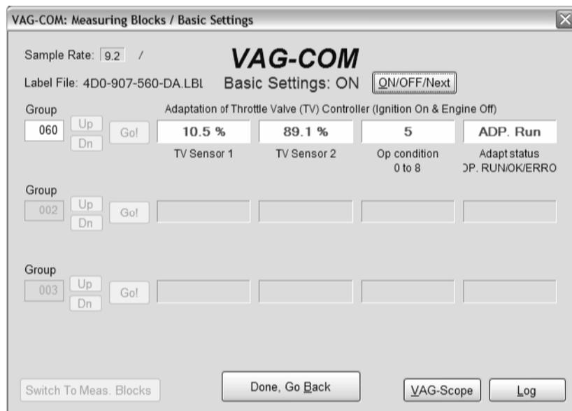
On Controllers using KWP-2000, there is an **[ON/OFF]** button that allows you to initiate and exit Basic Settings while still being able to see the values in the measuring groups.
