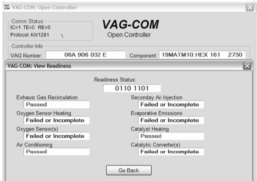
The above screen-shot was taken immediately after clearing the DTC's in a 2000 New Beetle 1.8T. You can see that this car does not support "monitors" for the EGR, Catalyst Heating, or Air Conditioning because this specific car does not have EGR or Catalyst Heating. It does have Air Conditioning, but a "monitor" is only required if the system uses ozone-depleting refrigerant (R12).
